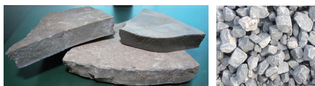
写真14 開発した低吸水性粗骨材の外観 Photo 14 Appearance of plate-like solidified slag and developed coarse aggregate
