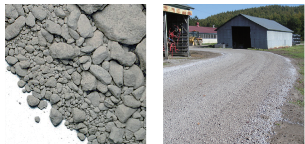
写真9 土工用製鋼スラグと農道での施工例 Photo 9 Steel slag crushed stone for civil engineering works and example of construction for farm road
